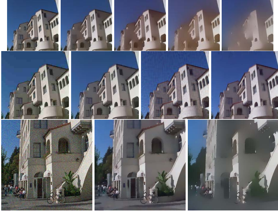
Fig. 4. Upper row: The Beltrami flow as an edge preserving scale space in color. Second row: Reconstructing a color image with noise artifacts introduced by wavelet lossy compression. The noisy image is on the left, the next image is the result of applying the Beltrami flow without constraints. Next is a reconstruction with noise artifacts introduced by JPEG compression. Again the noisy image is on the left and the reconstruction on the right Third row: Reconstruction of a color image corrupted with Gaussian noise; the second image is the result of flow with constraints (convergent scheme), while the third image is the result of the flow without constraints after the same number of numerical iterations. [This is a color image].
