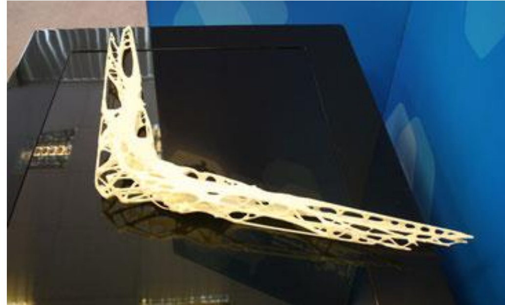
3D printed wing structure resembling the skeleton of birds
