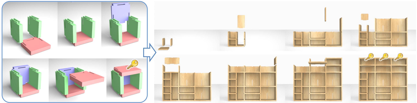
Fig. 15. Left: a single-key interlocking box assembled from three unique parts. Right: ARMOIRE composed of tileable boxes and three global keys on top.
