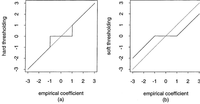
Fig. 4. (a) Hard and (b) soft thresholding rule for \lambda = 1
