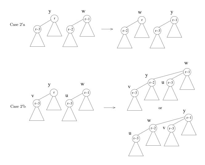
Figure 3: Alternative repair step for thin heaps. The outcome in Case 2'b depends on which of y and w has smaller key.
