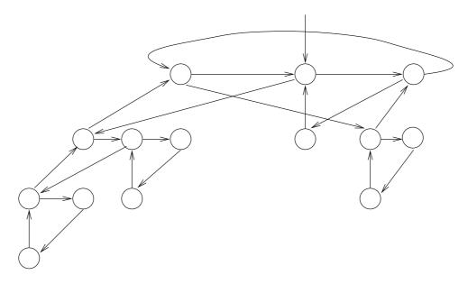
Figure 5: Two pointer-per-node representation of a heap. The heap consists of three binomial trees, a  $B_3$ , a  $B_1$ , and a  $B_2$ . This representation is essentially the reverse of Brown's "structure K".
