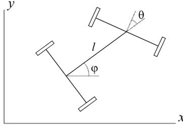
Fig. 5. Kinematic car model
