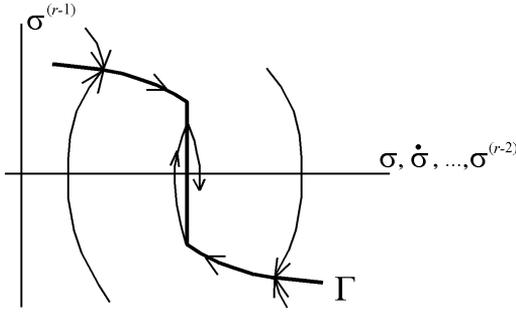
Fig. 2. The idea of  $r$ -sliding controller
