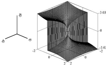
Fig. 3. The discontinuity set of the 3-sliding controller
