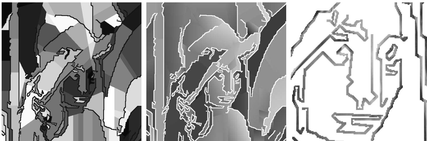
Fig. 6. (a) The final partition obtained with the convex-based dyadic partitioning, (b) its corresponding polynomial approximation, (c) the linear interpolation at the bands
