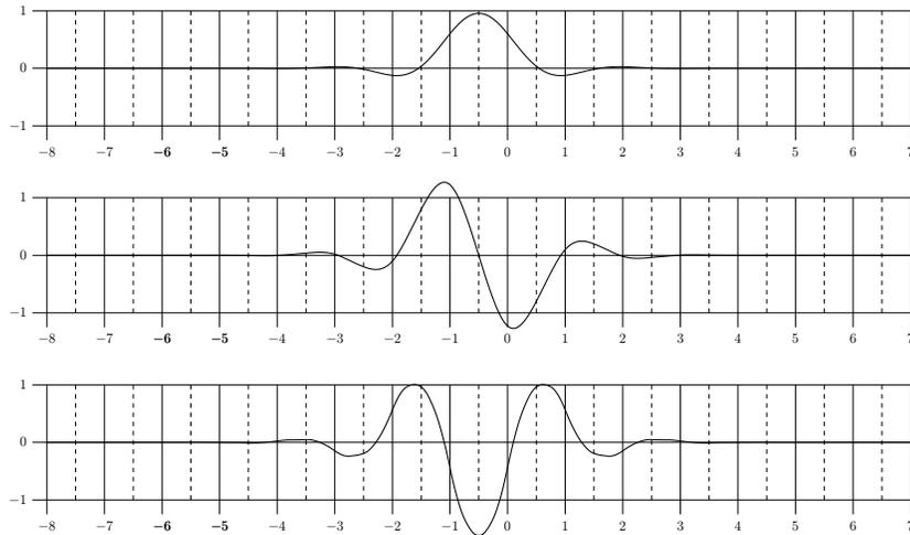
**Fig. 3.** Basic limit function of the new eight-point scheme, and its first and second derivative.
