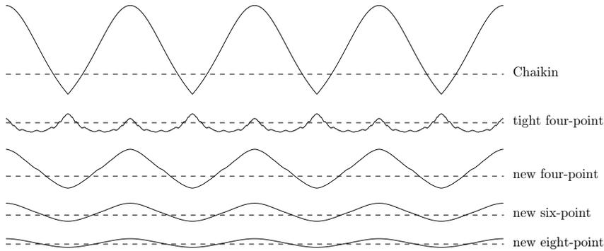
**Fig. 5.** Curvature plot of the curves in Figure 4. The dashed line indicates the curvature of the interpolating circle.
