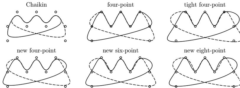
**Fig. 7.** Locality of the basis functions, visualized by moving the bottom left control point (full curve) to the right (dashed curve).
