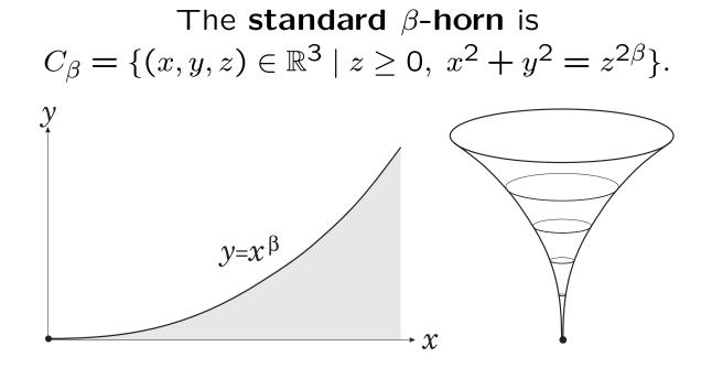
**Example.** A  $\beta$ -horn is a surface of revolution of a  $\beta$ -cusp  $x = y^{\beta}$ ,  $\beta \ge 1$ .
