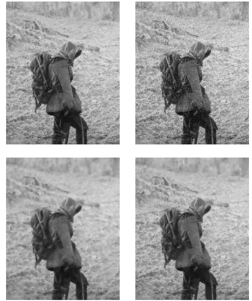
Fig. 7. Comparison between regularized Perona-Malik and our adaptive scheme. Top: original (left), image contaminated by additive white Gaussian noise (right, \sigma = 15 ). Bottom: image denoised using regularized Perona-Malik (P-M) (left) and processing with adaptive \lambda . Textures and small scale features are kept better in our scheme.
