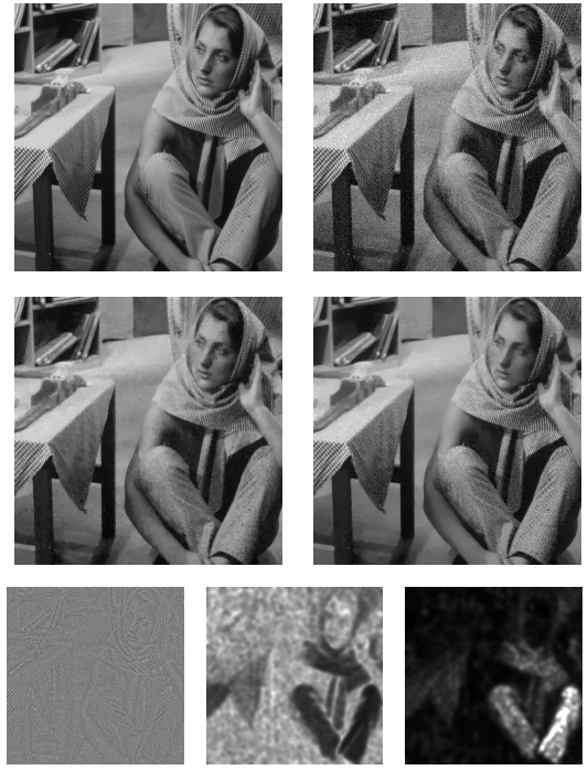
Fig. 4. An example of processing results obtained with a natural image. From top: Original 'Barbara image' (left); Noisy version of the original image, I_0 , with \text{SNR}=8.7\text{dB} , \sigma = 20 (right); Result of processing with scalar \lambda ( \text{SNR}=12.6\text{dB} , left); Result of processing with adaptive \lambda ( \text{SNR}=14.2\text{dB} , right); Residue I_R (left); S(x, y) calculated according to residue (middle); \lambda(x, y) at convergence of process (right).
