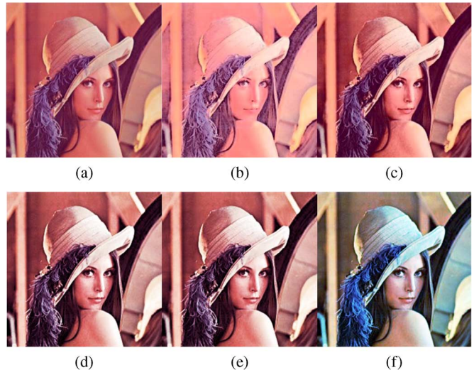
Fig. 6. Results of the histogram equalization on Lena. (a) Input image. (b) Result of Trahanias's method. (c) Result of Menotti's method. (d) Result of Naik's method. (e) Result of the proposed iso-luminance-plane method. (f) Equalized image of each RGB color channel.
