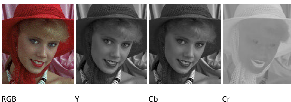
Figure 3. RGB to YCC Conversion - The original RGB image and the computed luminance (Y), chrominance-blue (Cb), and chrominance-red (Cr) images.
