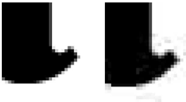
Figure 12. JPEG effects on line art - The image on the left is an original digital image of the serif on a lowercase "a". The image on the right shows the artifacts that are seen when this image is stored as a JPEG file with a user-specified quality factor of 20.
