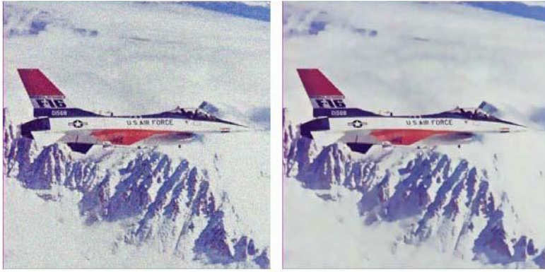
FIG. 11. NL-means denoising experiment with a color image. Left: Noisy image with standard deviation 15 in every color component. Right: Restored image.
