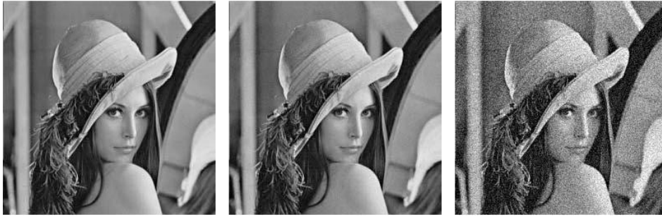
Fig. 1. A digital image with standard deviation 55, the same with noise added (standard deviation 3), the SNR therefore being equal to 18, and the same with SNR slightly larger than 2. In this second image, no alteration is visible. In the third, a conspicuous noise with standard deviation 25 has been added, but, surprisingly enough, all details of the original image still are visible.
