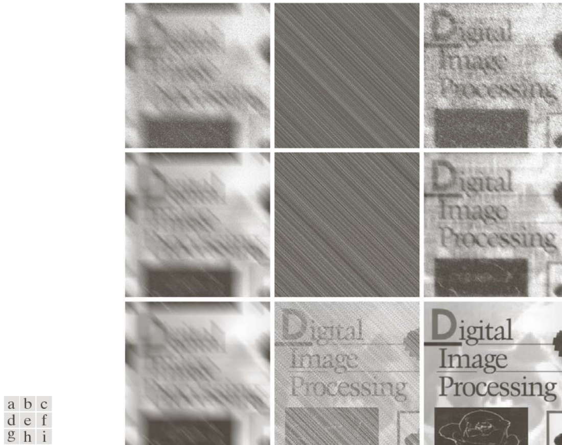
FIGURE 5.29 (a) 8-bit image corrupted by motion blur and additive noise. (b) Result of inverse filtering. (c) Result of Wiener filtering. (d)–(f) Same sequence, but with noise variance one order of magnitude less. (g)–(i) Same sequence, but noise variance reduced by five orders of magnitude from (a). Note in (h) how the deblurred image is quite visible through a “curtain” of noise.
