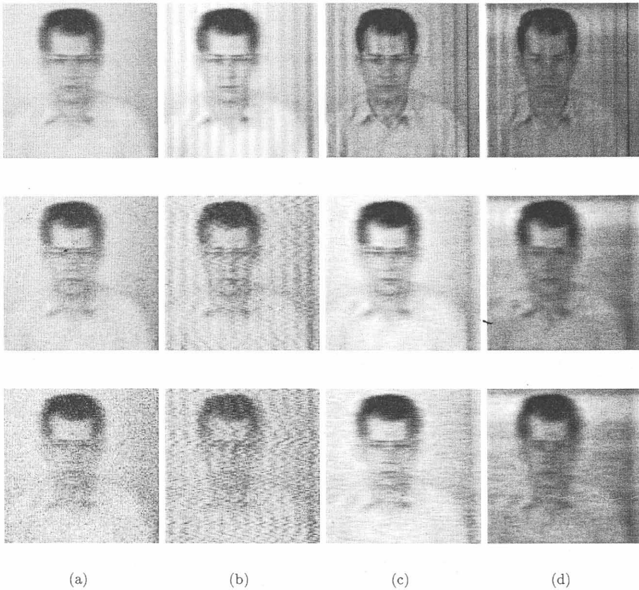
Figure 6.12: (a) Original images. (b) Restoration by inverse filtering with omission of all terms beyond the first zero of the filter transfer function. (c) Restoration by Wiener filtering. (d) Restoration by constraint matrix inversion.
