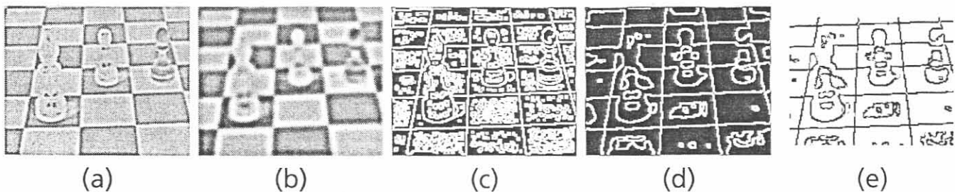
Figure 1.11 Steps in the computation of the Marr-Hildreth edge detector. (a) Convolution of the original image with the Laplacian of a Gaussian having \sigma = 1.2 . (b) Convolution of the image with the Laplacian of a Gaussian having \sigma = 2.8 . (c) Zero crossings found in (a). (d) Zero crossings found in (b). (e) Result, found by using zero crossings common to both.
