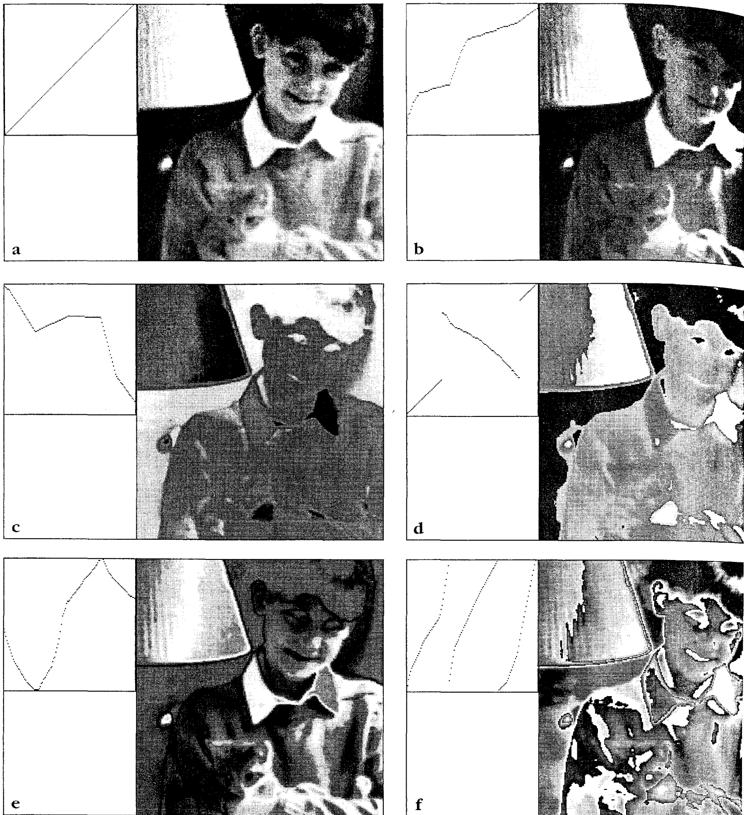
Figure 1. An original image with a full range of brightness values and several examples of arbitrary hand drawn display transfer functions which expand or alter the contrast in various parts of the range. The plot with each image shows the stored pixel brightness values on the horizontal axis and the displayed brightness on the vertical axis. Image a) has a transfer function that is the identity function, so the actual stored brightnesses are displayed. Images b) through f) illustrate various possibilities, including reversal and increased or decreased slope over parts of the brightness range.
