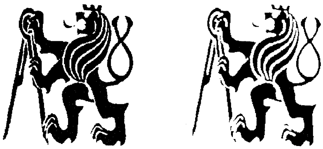
Figure 11.8: Erosion as isotropic shrink.
