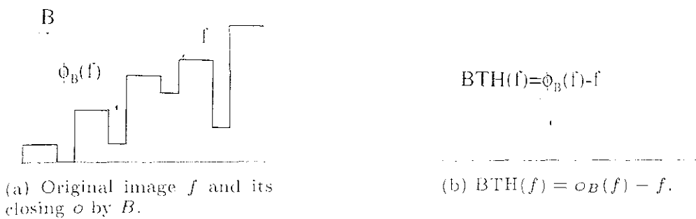
Fig. 4.16. Black top-hat BTH performed on a 1-D signal. Note that the troughs are extracted independently of their intensity levels.
