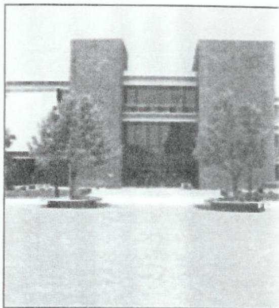
b. Result of Y_p mean filter on image with salt noise; mask size = 3, order = -3.
