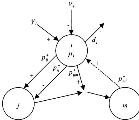
Fig. 3. Some of the possible stochastic transitions and their rates and probabilities, occurring at queue  $i$ . A plus sign is written beside transitions that increase the length of the target queue; a minus sign denotes transitions that decrease the length of the target queue. Note that these transitions apply to each queue in the network; as an example, one of the transitions occurring at queue  $m$  is depicted (the dashed arrow).
