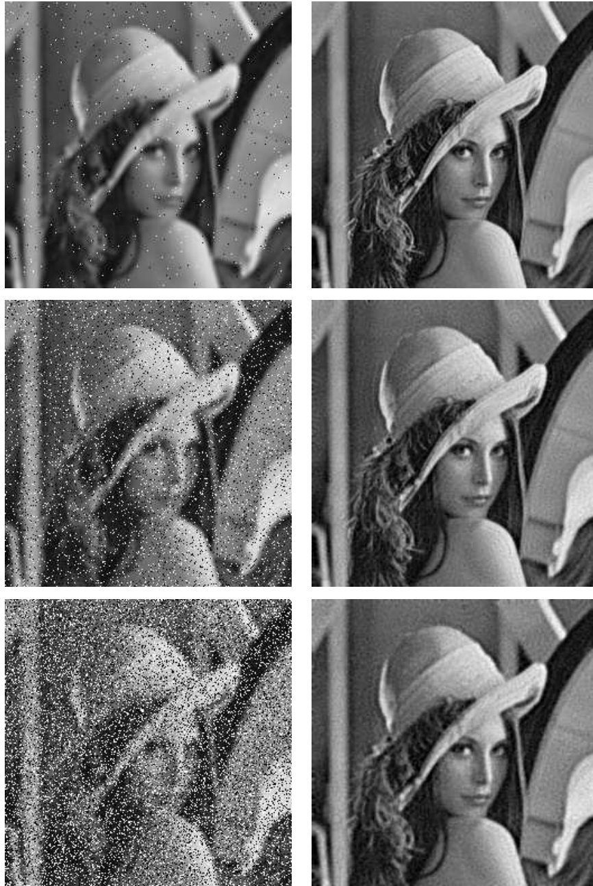
Figure 6: Left column: The Lena image, blurred with a pill-box kernel of radius 3, and contaminated by salt and pepper noise. The noise densities are (top to bottom) 0.01, 0.1 and 0.3. Right column: The corresponding recovered images.
