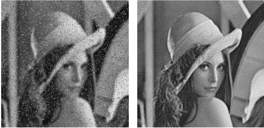
Figure 8: Deblurring in the presence of random impulsive noise. Left: Source image, blurred with a pill-box kernel and contaminated by random impulse noise of 0.1 density. Right: Recovered image, using the suggested algorithm.
