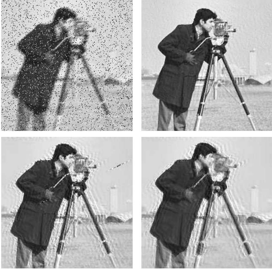
Figure 7: The case of motion blur. Top-left : Blurred and noisy image. Top-right : Restoration using the proposed method. Bottom-left : The outcome of 3 \times 3 median filtering followed by TV [38] restoration. Bottom-right : The outcome of 5 \times 5 median filtering followed by TV [38] restoration.
