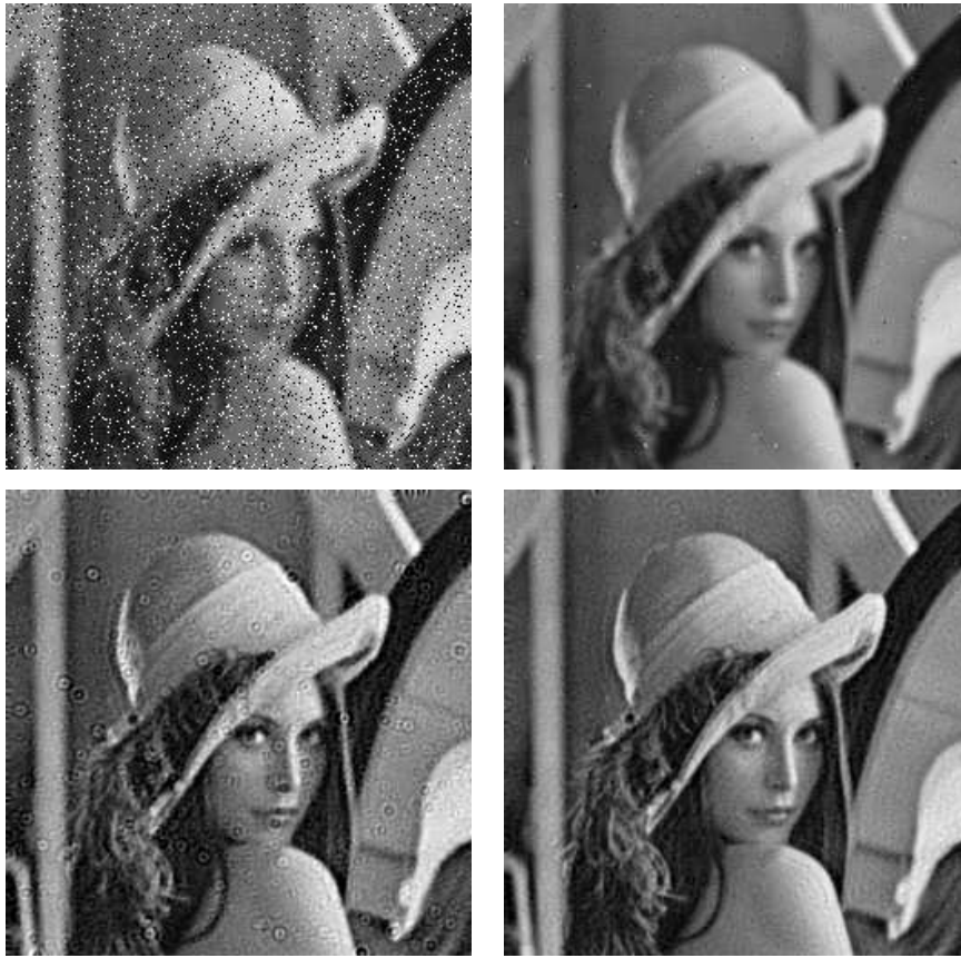
Figure 9: Deblurring in two stages. Top-left : Source image, blurred with a pill-box kernel of radius 3, and contaminated by noise of density 0.1. Top-right : Denoised image by Mumford-Shah method Bottom-left : TV Deconvolution of the denoised image Bottom-right : Recovered image using the suggested algorithm
