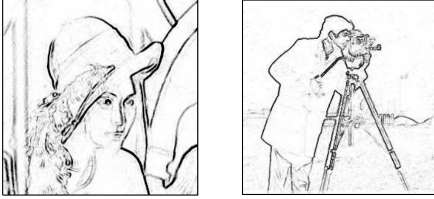
Figure 13: Approximated edge maps obtained as a by-product of the restoration process. Left: The v -function that corresponds to the deblurring of the Lena image with a pill-box kernel and noise density 0.1. Right: The v -function that corresponds to the deconvolution of the Cameraman image with motion-blur and noise density 0.1.
