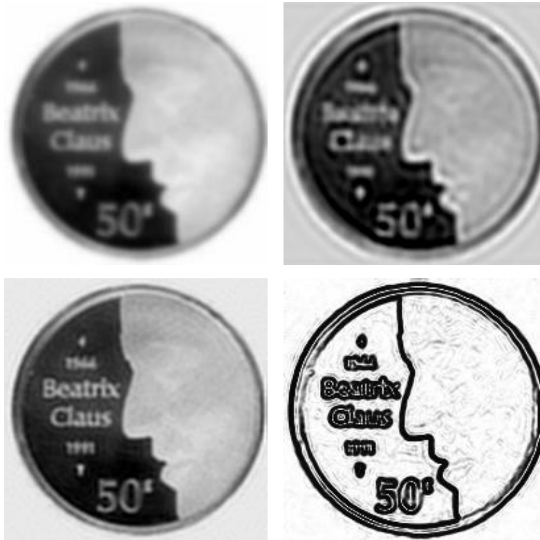
Fig. 5. Segmentation and blind restoration. Top-left: Blurred ( \sigma = 2.1 ) image with slight additive noise. Top-right: Restoration using the method of [6]. Bottom-left: Restoration using the suggested method. Bottom-right: Edge map produced by the suggested method.
