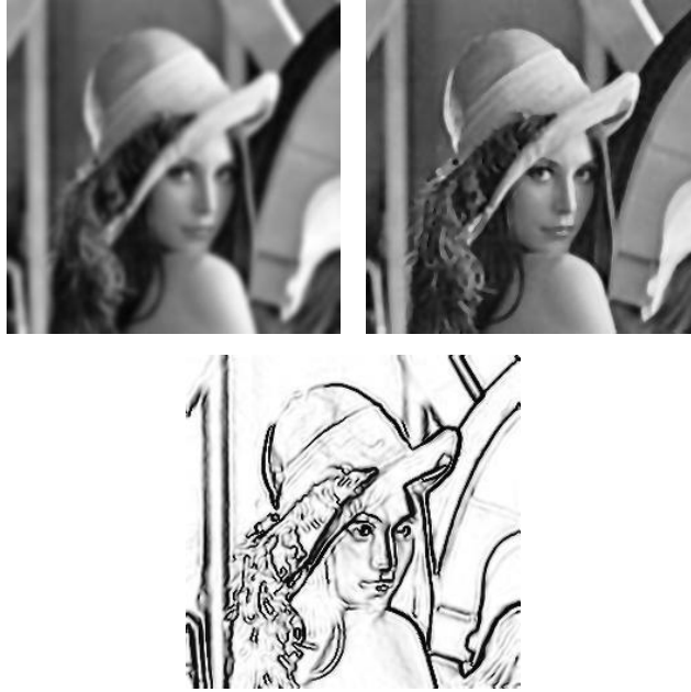
Fig. 4. Segmentation and blind restoration. Top-left: Blurred image ( \sigma = 2.1 ). Top-right: Blind reconstruction using the proposed algorithm. Bottom: Edge map v produced by the suggested method. Compare to Fig. 1.
