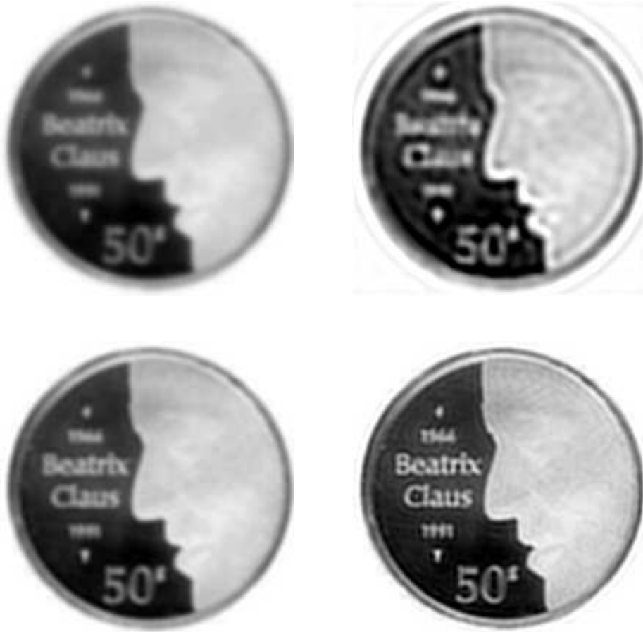
Figure 5: Semi-blind restoration. Top-left : Blurred ( \sigma = 2.1 ) image. Top-right : Restoration using the method of [8]. Bottom-left : Restoration using a modified version of [8], in which the kernel was restricted to the family of isotropic Gaussians. Bottom-right : Restoration using the method suggested in this paper.
