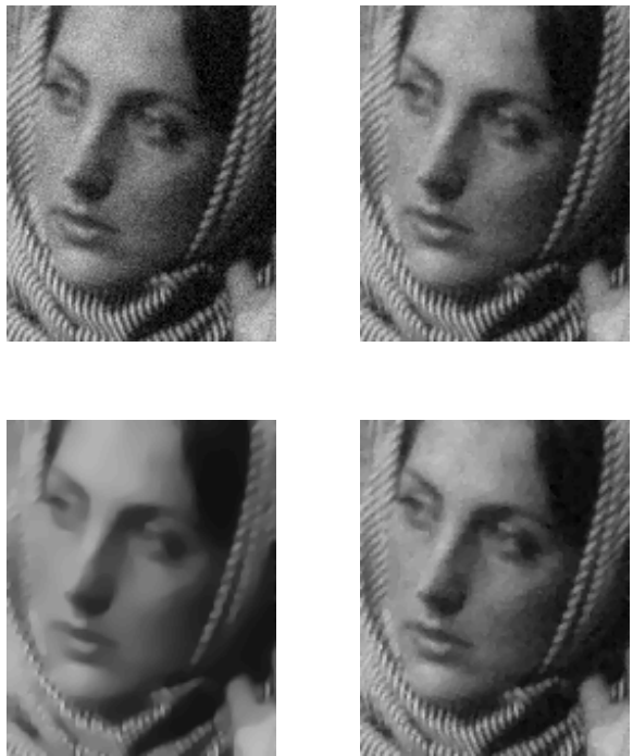
Fig. 13. Effects of stopping criterion on processing results of different stopping times, processing Barbara image (head part is shown). Top left: noisy image f ; Right - Weickert’s method (24). Bottom left: Mrazek-Navara (23), right - our method of direct estimation.
