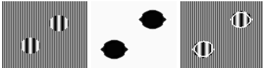
Fig. 2. a. A synthetic image made up of 2D sinewave gratings containing background and object of different scales (left). b. The stopping function E (middle). c. The resultant boundary(right).
